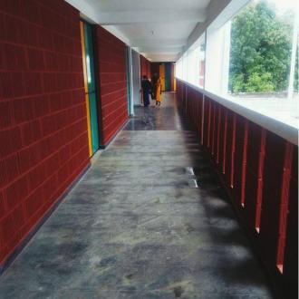
This is the largest project for OSAAT so far, in terms of the budget – here we constructed a new building with 8 classrooms, staff rooms and toilets. Construction was done using hollow clay blocks by Porotherm Smart Bricks. These blocks are designed to provide better efficiency, durability, ease of use and a host of other benefits that aid in cost- effective wall construction.
